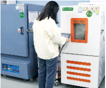
Constant Temperature & Humidity Tester
