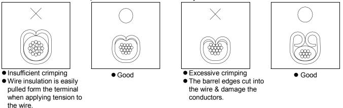
Check: Cut off the insulation support and remove the wire insulation, then check the wire conductors for damage.
